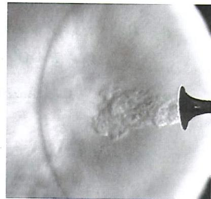
Fig 2. Schlieren image showing shock wave from a Trumpet.
